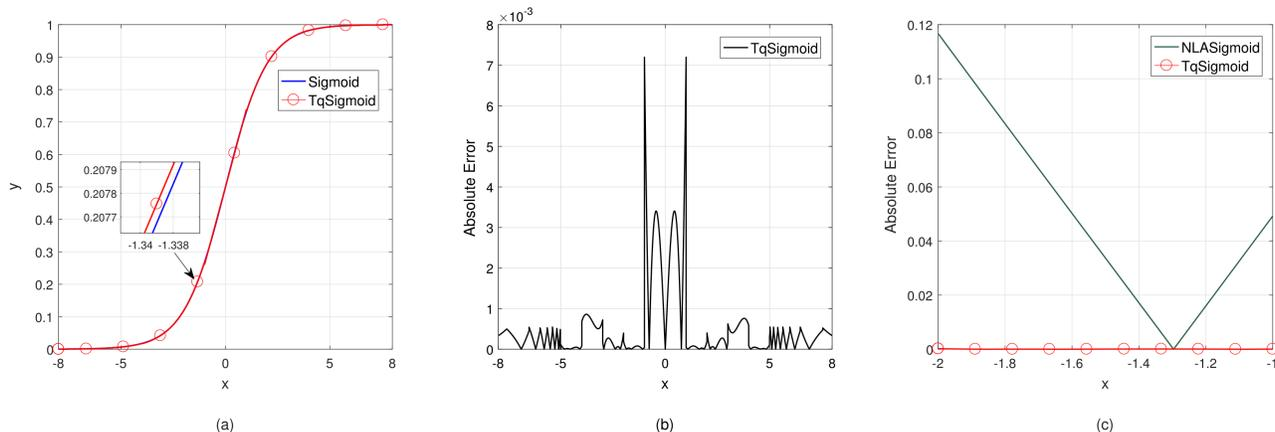
Fig. 3. Evaluation results of the approximate sigmoid function: (a)  $TqSigmoid$  and the sigmoid function (b) absolute error of  $TqSigmoid$  (c) absolute error of  $NLASigmoid$  [16] and  $TqSigmoid$  in the piece-wise interval of  $[-2;-1]$ .
