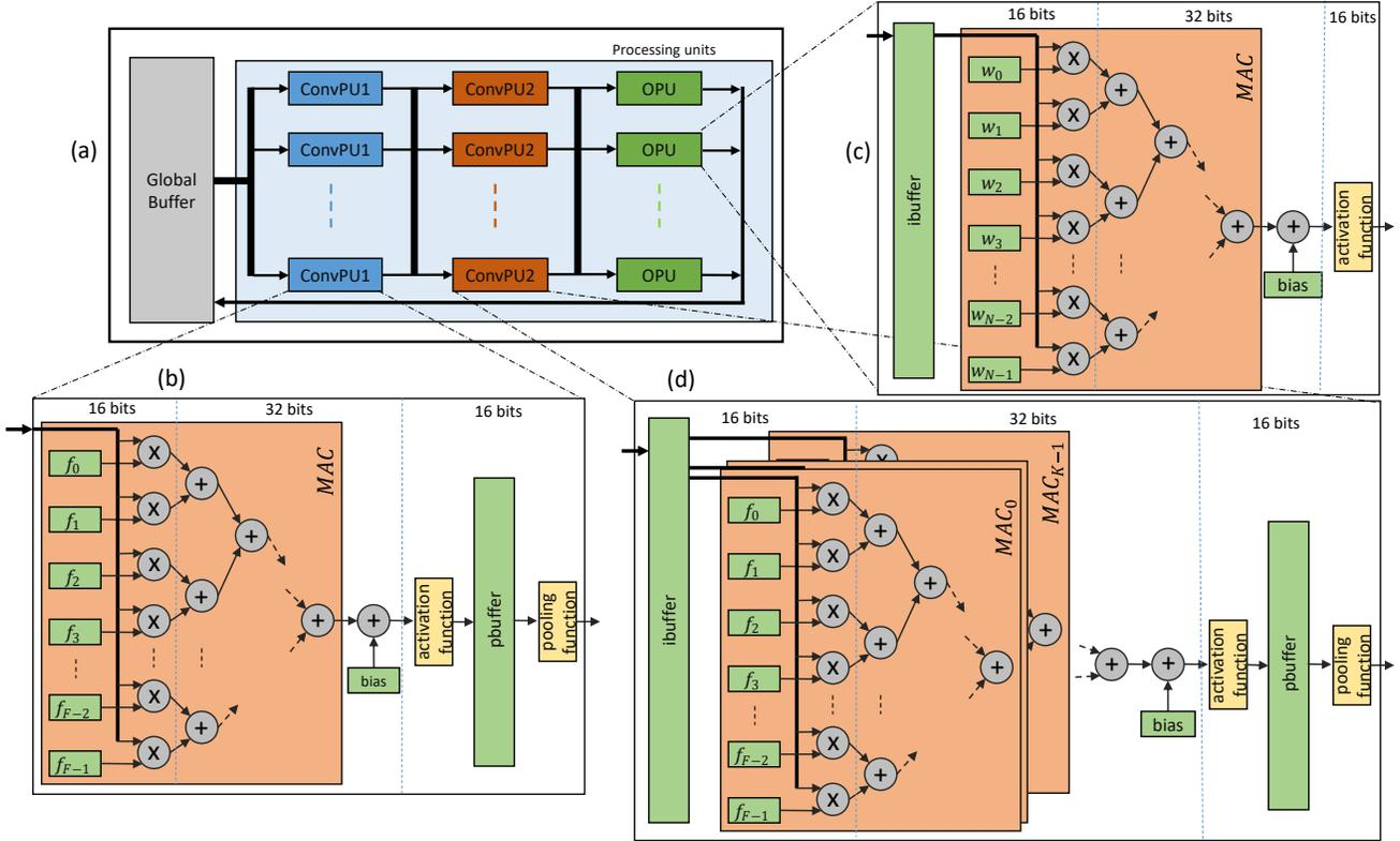
Fig. 1. NASH-CNN system architecture.
